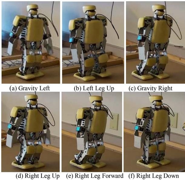
Figure 2. Configurations of the robot walking forward behavior
