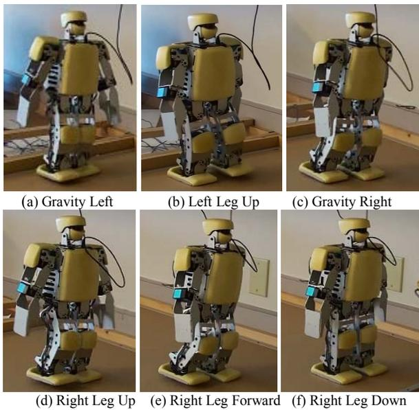
Figure 2. Configurations of the robot walking forward behavior
