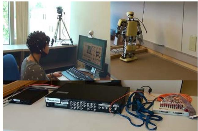
Figure 1. BCI-based humanoid robot control system
