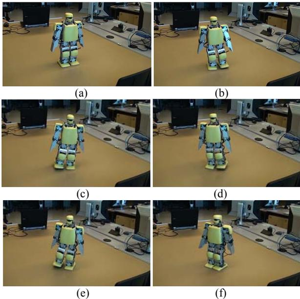
Figure 6. Control of robot turning left through brainwaves
