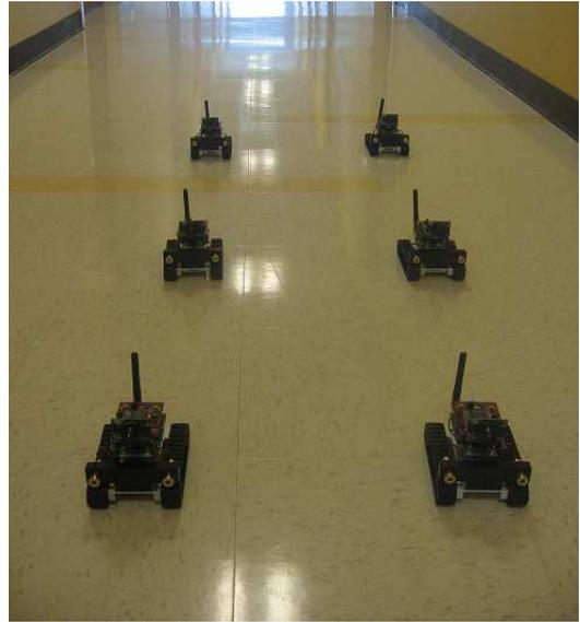
Fig. 6: A fleet of Surveyor's SRV-1 internet-controlled robots with wireless communication is chosen for the tracing of multiple plumes.
