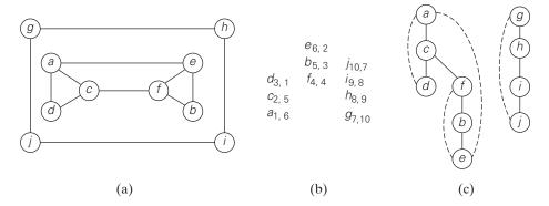
**FIGURE 3.10** Example of a DFS traversal. (a) Graph. (b) Traversal's stack (the first subscript number indicates the order in which a vertex is visited, i.e., pushed onto the stack; the second one indicates the order in which it becomes a dead-end, i.e., popped off the stack). (c) DFS forest with the tree and back edges shown with solid and dashed lines, respectively.
