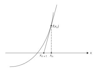
FIGURE 12.22 Iteration of Newton's method.
