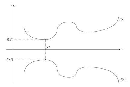
**FIGURE 6.17** Relationship between minimization and maximization problems:  $\min f(x) = -\max[-f(x)].$
