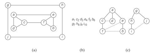
**FIGURE 3.11** Example of a BFS traversal. (a) Graph. (b) Traversal queue, with the numbers indicating the order in which the vertices are visited, i.e., added to (and removed from) the queue. (c) BFS forest with the tree and cross edges shown with solid and dotted lines, respectively.
