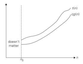
**FIGURE 2.2** Big-omega notation:  $t(n) \in \Omega(g(n))$ .
