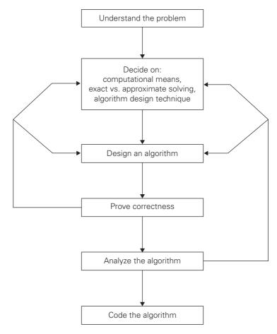
FIGURE 1.2 Algorithm design and analysis process.
