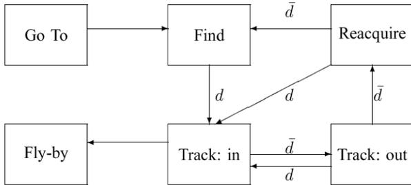
**Figure 2.** Behavior Switching Diagram. The symbol  $d$  denotes a behavior switch that occurs when chemical is detected. The symbol  $\bar{d}$  denotes a behavior switch that occurs when chemical is not detected for some time interval.
