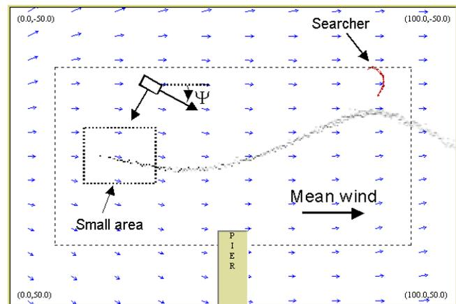
**Figure 1.** Depiction of a vehicle (not to scale) performing chemical plume tracing. The array of blue arrows indicate the direction and relative magnitude of the flow at the tail of the arrow. The numbers in the four corners are the coordinates of the corners. The meandering gray-scale trail is the plume. The chemical source is at (20,0) m. The start of the searcher trajectory is the curved red path in the upper right.
