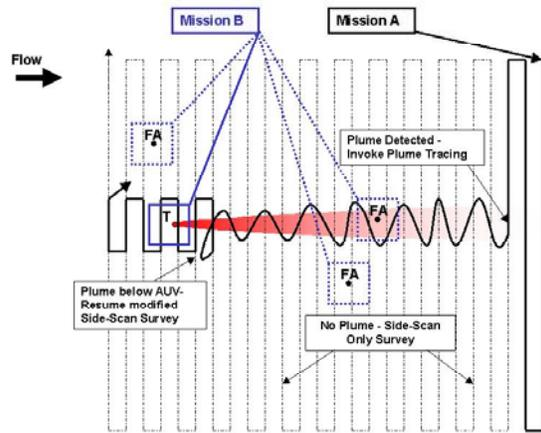
Figure 7. A prototype CPT mission with Flyby.
